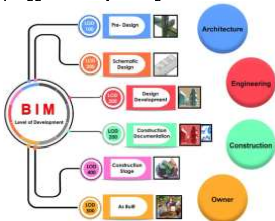
Gambar 9. The Level of Development (LOD) Specification is a reference that enables practitioners in the AEC Industry to specify and articulate with a high level of clarity, the content and reliability of Building Information Models (BIMs) at various stages in the design and construction process (Scriinsoft Inc, 2019)
